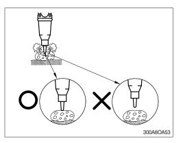
Move the impact point from the edge to the interior. Never try to break off a too large block, if the object has not broken within 30 seconds. The object should be broken up piece by piece in small blocks. Large distance steps will not improve working results.
